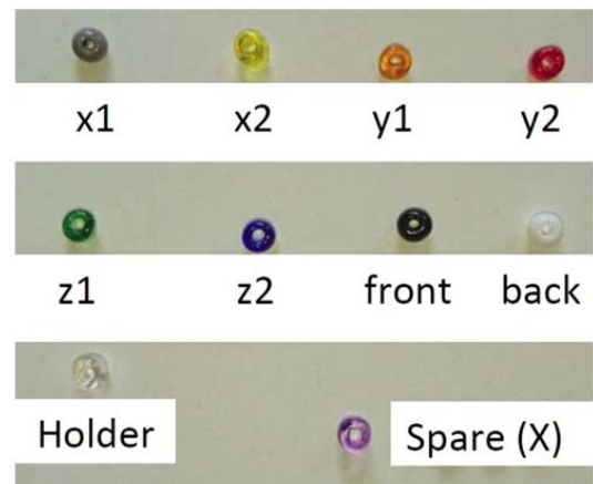
Figure 2.4: In-vacuum cable color code
