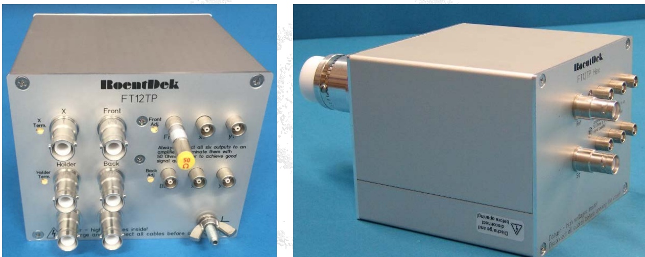
Figure 2.5: FT12TP plug for DLD with rectangular case and 50 Ω terminator, here placed on MCP front output (MCP back output can thus be used for MCP signal pickup)
