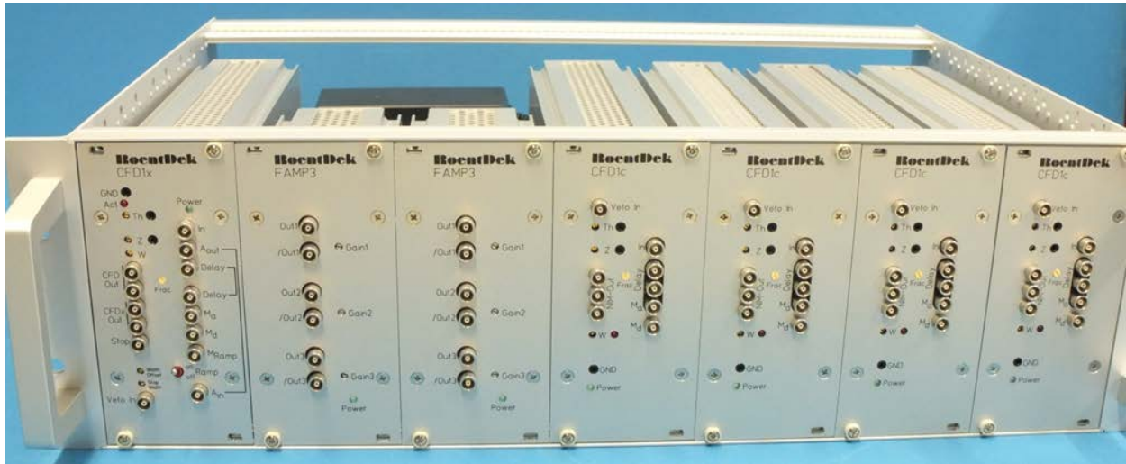
Figure 3.3: with 19" 3HU crate hosting six amplifier channels (FAM6L or two FAMP3) and 4+1 CFD channels (four CFD1c plus one CFD1x). The CFD1x has additional circuits to transform pulse height information into a time delay for recording by a TDC channel. Below: version FEE5 with CFD4L (replacing four CFD1c) and standard CFD1c (can also be upgraded to FEE5x). For cabling please refer to the FEE5 connection scheme .
