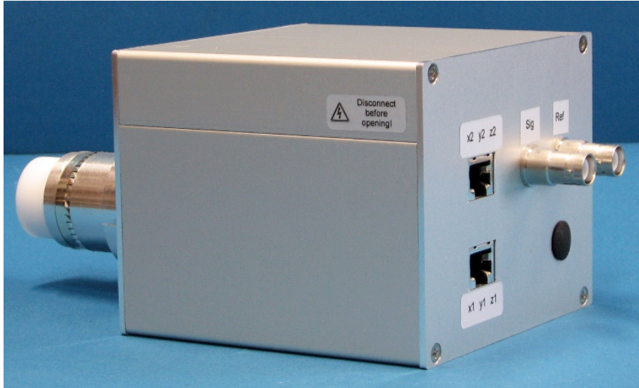
Figure 2.6: FT12TPhex plug with rectangular case, here with differential signal output via CAT6 cables
