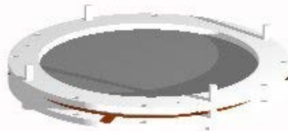
Figure 1.14: Assembly of MCP stack - Stage 3-1 (DLD40, DLD80 & HEX80)
