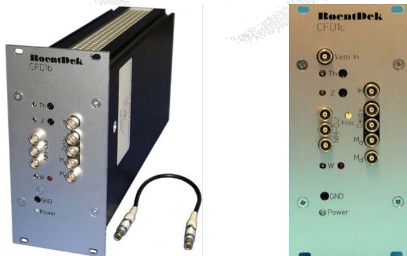
Figure 3.2: Single-channel constant fraction discriminator CFD1c for retrieving the time information of fast signals off an MCP detector or similar devices.
