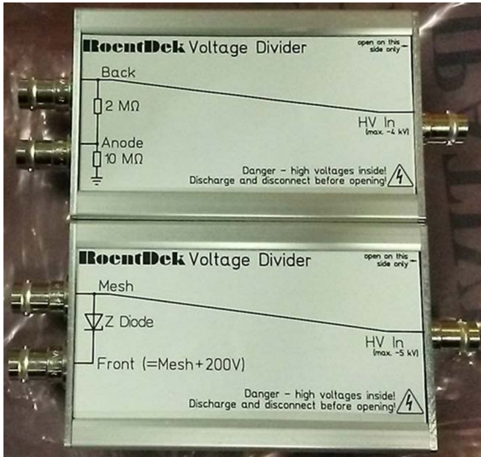
Figure 5.27: Set of voltage divider boxes for DET operated at high negative bias (MCP front up to -4800 V) with a mesh biased 200 V more negative than MCP front (lower box) and a resistor divider chain for biasing MCP back and Anode at adequate potential for single particle counting (upper box). The voltage drop between MCP back and Anode is 1/6 of the MCP back potential, here (can be altered by changing the 2 MΩ resistor, see Kirchhoff's laws).
