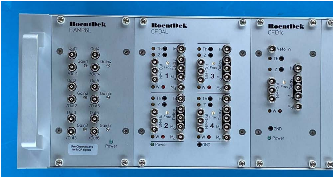
Figure 3.3: with 19" 3HU crate hosting six amplifier channels (FAM6L or two FAMP3) and 4+1 CFD channels (four CFD1c plus one CFD1x). The CFD1x has additional circuits to transform pulse height information into a time delay for recording by a TDC channel. Below: version FEE5 with CFD4L (replacing four CFD1c) and standard CFD1c (can also be upgraded to FEE5x). For cabling please refer to the FEE5 connection scheme .
