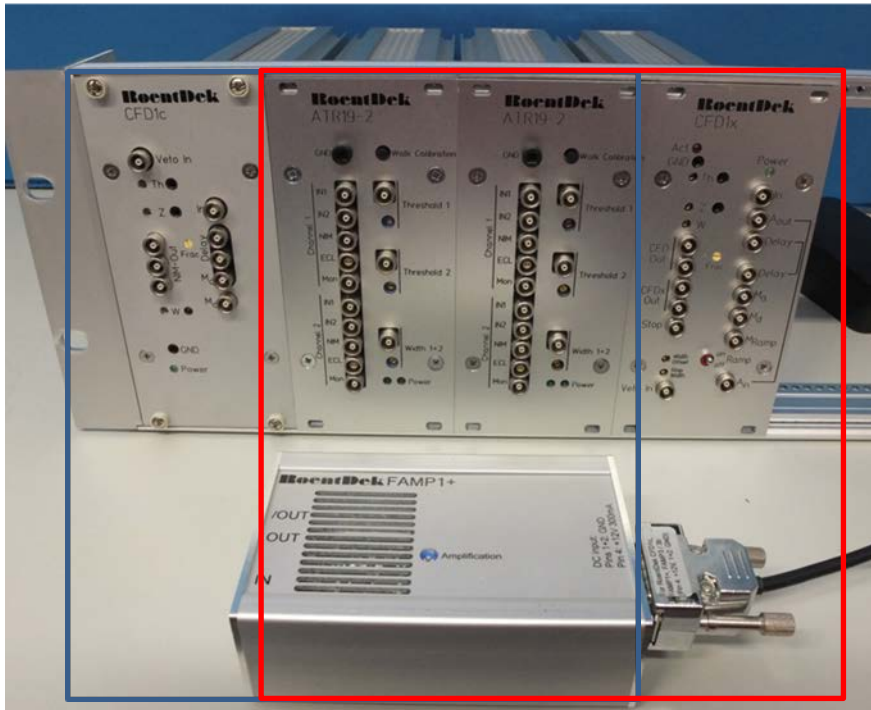
Figure 3.4: left picture: front side of FEE2 product assembly mounted in a 19" 3HU frame, three modules plus FAMP1+. The blue rectangle shows the items of the standard version with CFD1c, which can be replaced by a CFD1x (version FEE2x, in red rectangle). Upper picture: rear side view with loop through cable connections. The FAMP1+ module is also available as 3HU unit for rack mounting.
