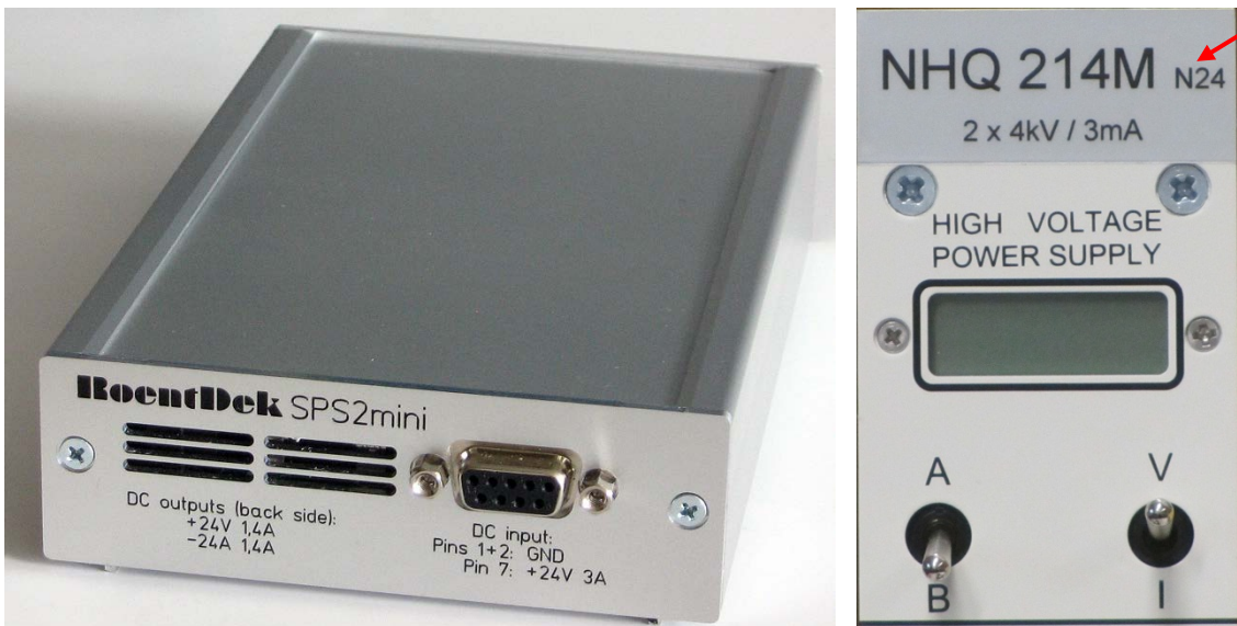
Figure 5.9: SPS2mini mains adapter (left) and the specific label (red arrow) on the front side of a “N24”- type HV2/4 module which can be powered by it (those units with side panel labels will show the N24 indication there).
