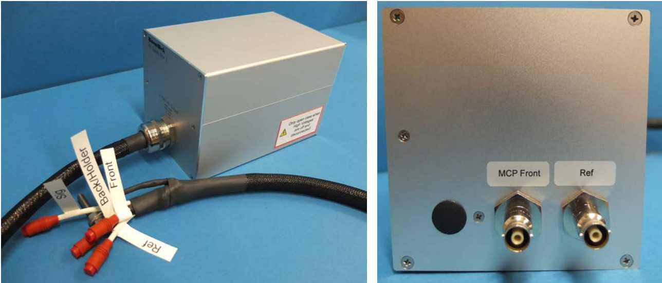
Figure 5.20: Left picture: HVZ10 box with four-fold high voltage output cable which will be connected to an XHV feedthrough. Right picture: high voltage inputs on rear panel. Here, two SHV10 socket are provided for supplying two independent voltages. Other versions are available which operate with just one input voltage (MCP front or U_{ref} ) and/or use other input socket standards
