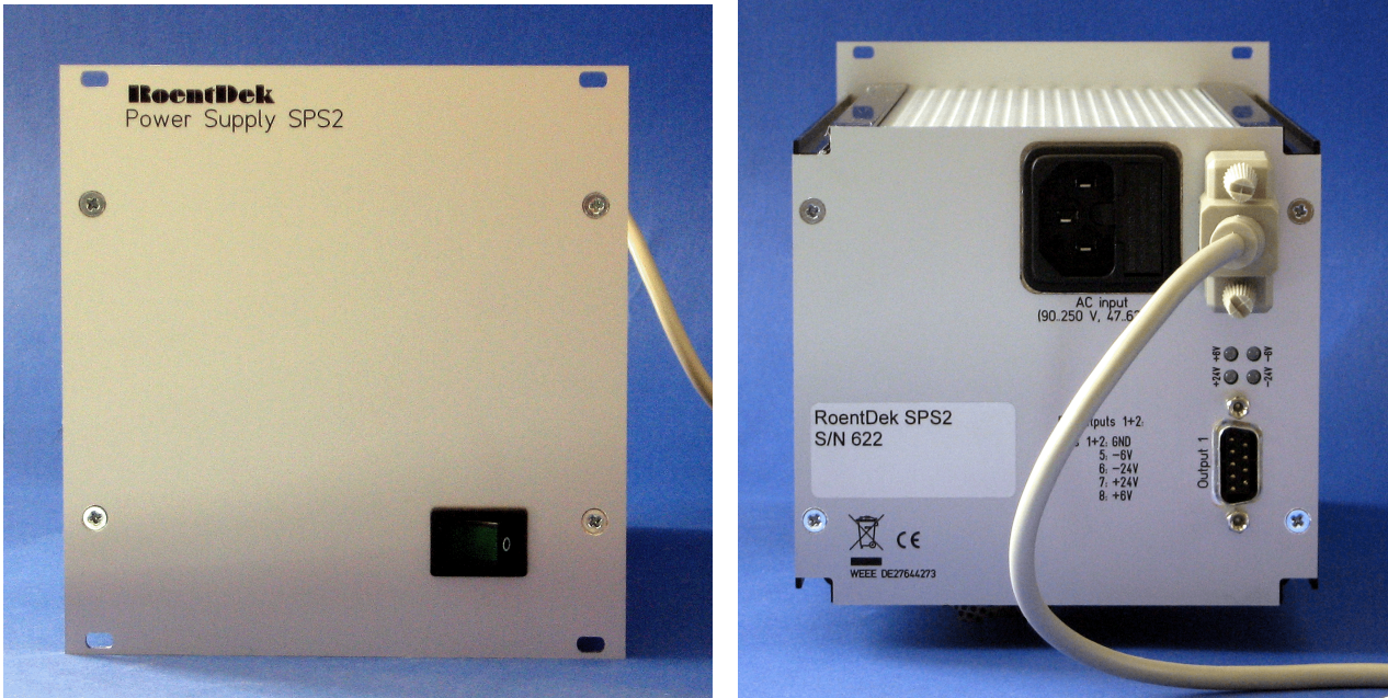
Figure 5.8: SPS2 front and rear panel with connection cable to HV2/4 module (not shown).
