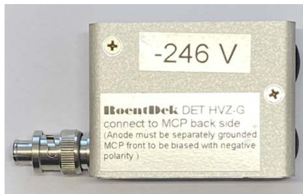
Figure 5.17 HVZ-G plug, here the version for negative bias of MCP back potential.
