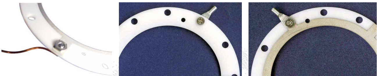
Figure 1.8: Connections to a ceramic ring. Left: cable clamped to a “front” ring. Middle/right: cable clamped to a back ring with 3 mm lug, countersunk M2 screw and special M2 nut.
